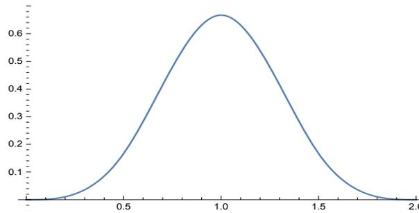
**Figure 4:** The *BSf* shapes with 3 degree is really  $\beta^3(t)$ .
